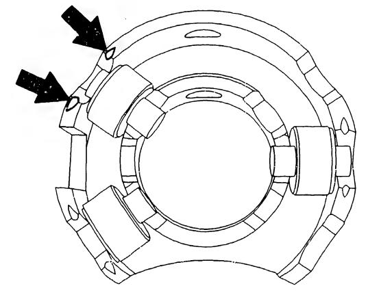
When installing the rollers, make sure that the spring seats are installed on the outside of the rollers.
